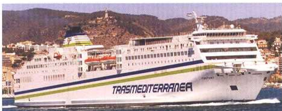
Trasmediterranea's 2001-built superferry Fortuny , which has been suffering from severe propeller-induced vibrations in the off-design condition, has recently been retrofitted with CLT high-skew CP propeller blades. The project marks a new era in the evolution of the CLT tipped design.
