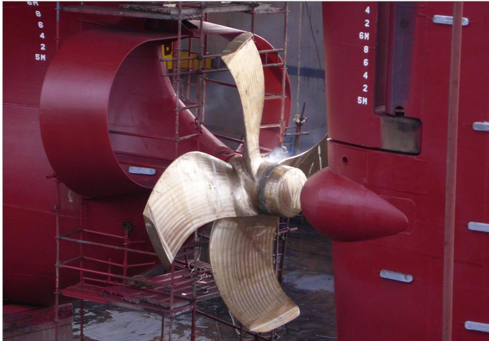
Figure 8. 35K DWT product tanker “Roy Maersk”, the retrofitted CLT propeller with pre-existing WED and bulbed rudder.
