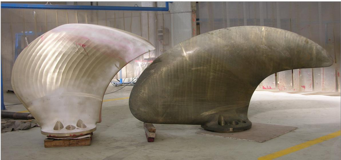
Figure 3. The striking difference between a CLT and a state-of-the-art high skew conventional propeller blade designed for the same Ro-Pax vessel and for the same speed
