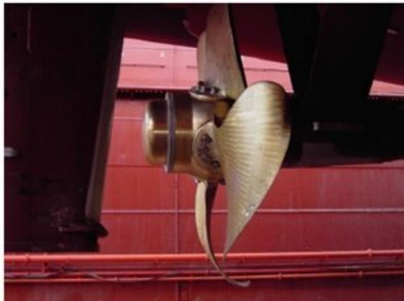
Figure 6. A CP Kappel propeller, note the winglet integrated in the blade and curling toward the suction side.
