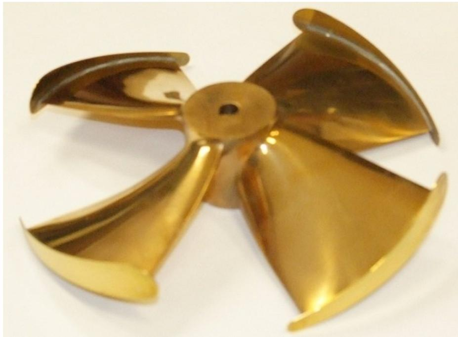
Figure 2. A TVF propeller blade and end plate.
