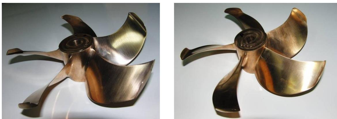
Figure 10. SISTEMAR CLT propeller, left, and NSWCCD TLP propeller, right. Albeit independently designed the two propellers are very similar.
