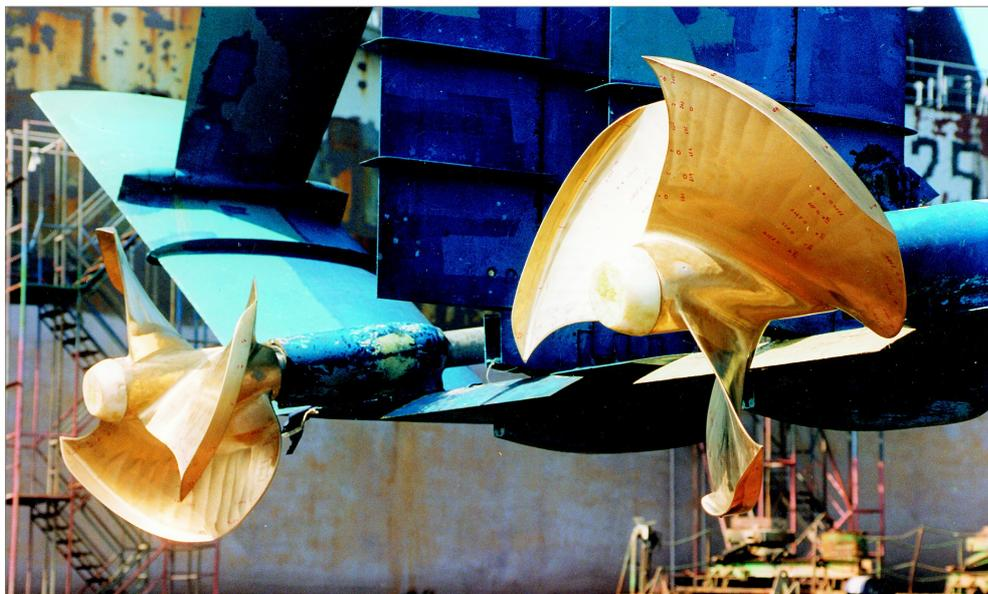
Figure 4. FP CLT propellers installed on an hydrofoil.
